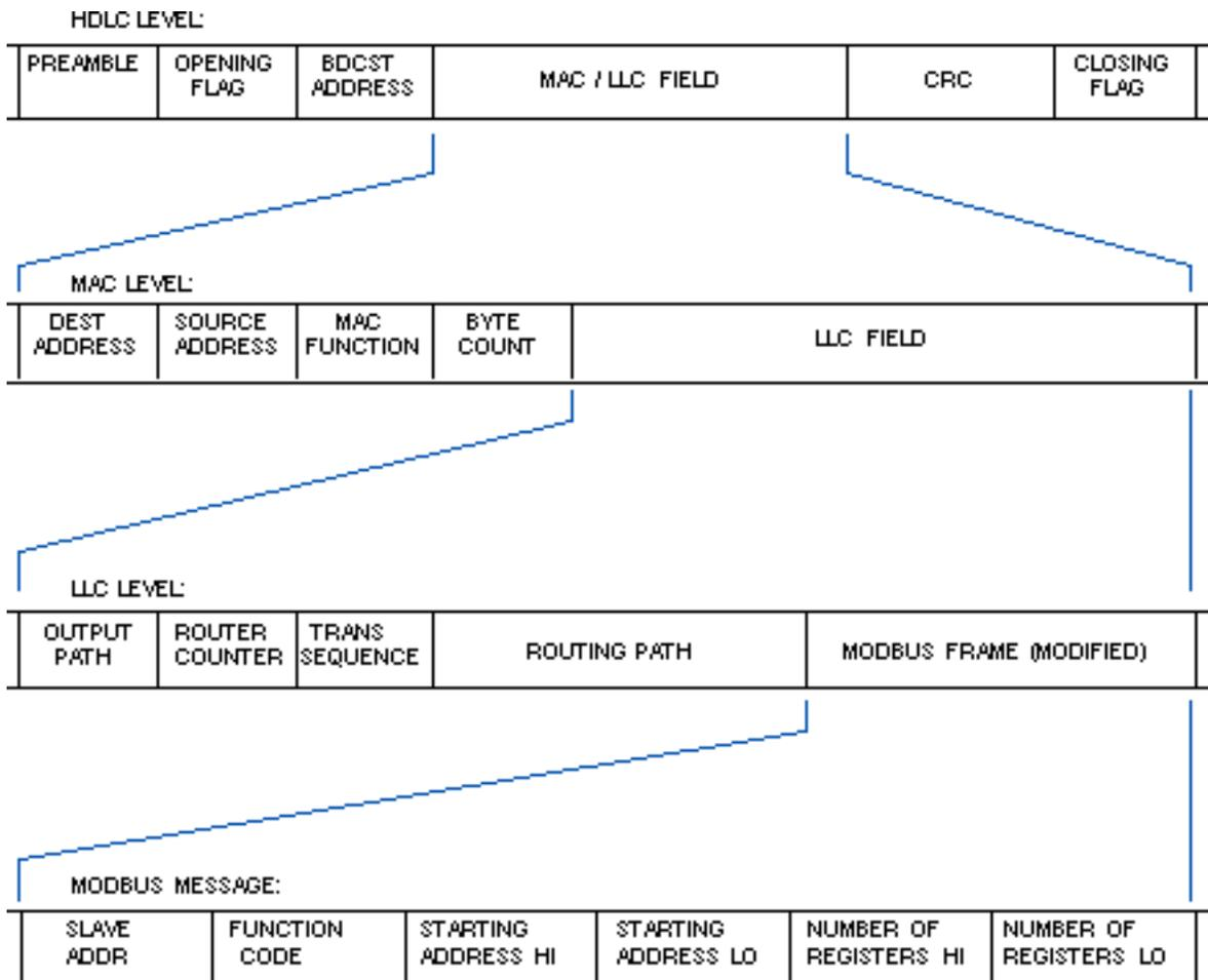
**Figure 7 Field Contents on Modbus Plus**
