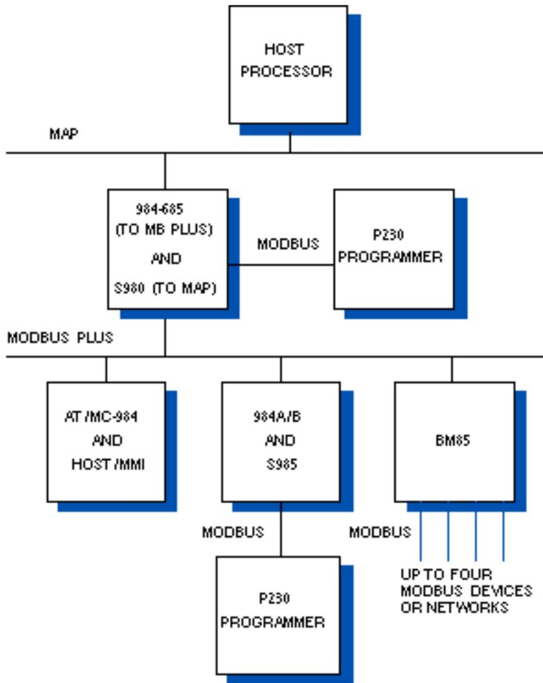
**Figure 1 Overview of Modbus Protocol Application**
